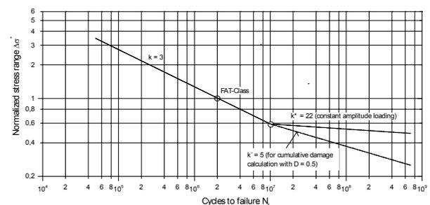
Fig. 4 - IIW-design curve for thick walled or stiff structures
