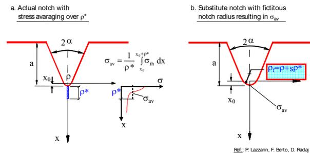
Fig. 2 - Neuber's microstructural concept
