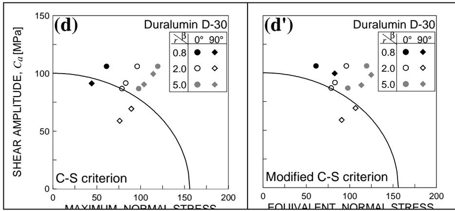
**Figure 2** Shear stress amplitude against maximum normal stress (diagrams (a) to (d)) and equivalent normal stress amplitude (diagrams (a') to (d')) acting on the critical plane: theoretical evaluations according to both the original or modified C-S criterion, and experimental results [20].
