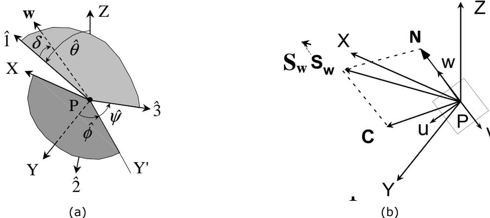
**Figure 1** (a) Correlation between averaged principal stress axes and normal  $w$  to the critical plane; (b) Stress components acting on the critical plane and  $\{Puvw\}$  local coordinate system ( $u$  and  $v$  belong to the critical plane).
